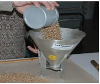
2.) Ensure the slide is inserted into the Cox funnel. Pour the contents of the 0.5 litre measure, plus an extra handful, into the Cox funnel.
