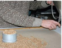
1.) Fill the 0.5 litre measure to overflowing with the grain to be tested.
