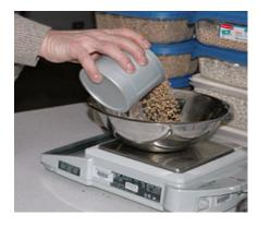
6.) Pour the grain remaining in the 0.5 litre measure into the scale pan. Determine the weight in grams of the grain in the scale pan. Convert the grams in the 0.5 litre measure to kilograms per hectolitre (kg/hl).
