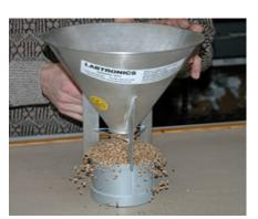
3.) Place the 0.5 litre measure on a solid base. Position the Cox funnel on top of the 0.5 litre measure so that the notched legs of the Cox funnel fit securely onto the measure's rim. Remove the slide on the Cox funnel quickly so that the grain drops evenly into the 0.5 litre measure.
